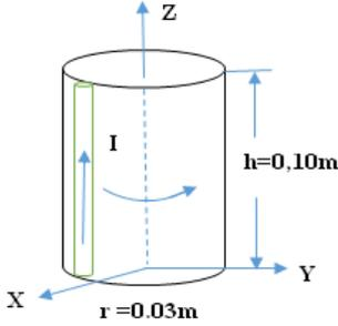
$$\vec{F}_a = I * (\vec{L} \wedge \vec{B}) = I * (L \cdot \vec{k} \wedge B \vec{e}_r) = 1.13 * 10^{-2} \vec{e}_\phi \text{ Newton}$$
